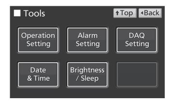
**4.** On the Date & Time screen, input the present date and time. Press Apply key to save the input value. The display returns to the Tools screen.
