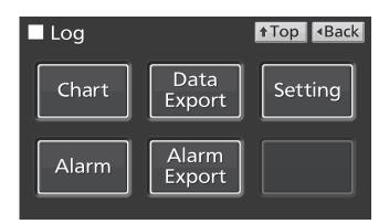
**4.** On the Setting screen, input Log Interval. Press Apply key to save the input value. The display returns to the Log screen.
