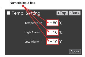
**2.** Press Numeric key or Up/Down key to input numerical value, and press OK key.
