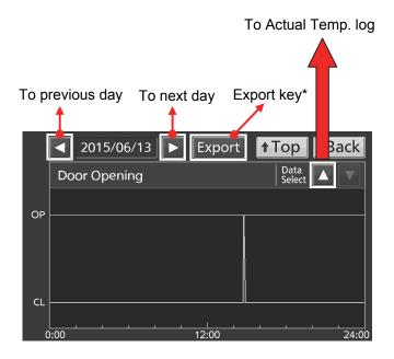
\*When exporting operation log data, without pressing the Export key, follow the procedure on page 34~36. When pressing Export key by mistake, press the Back key to return to the previous screen.
