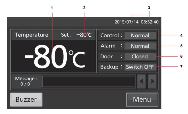
1. Present temperature display field: The current chamber temperature is displayed.
